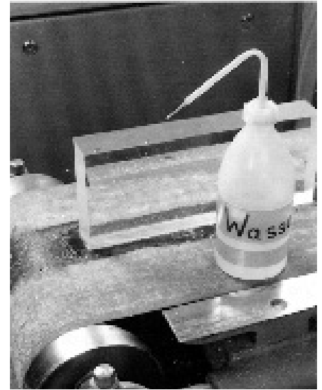
Fig. 38: Wet sanding on a belt sanding machine
