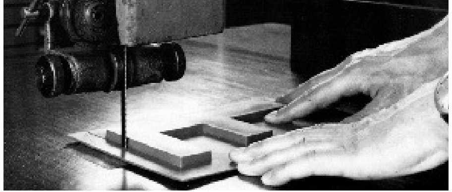
Fig. 7: Edge trimming with bandsaws
