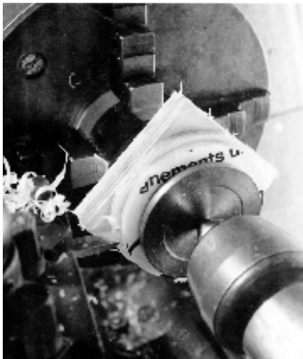
Fig. 30: Turning blanks into round discs between chuck and tailstock
