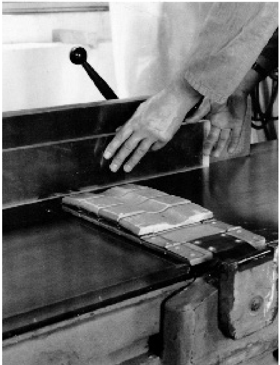
Fig. 36: Smoothing the edges with a surface planer
