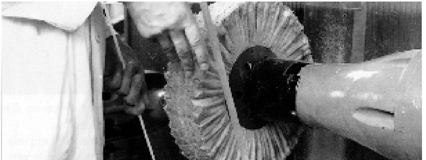
Fig. 40: Polishing against a cloth buffing wheel
