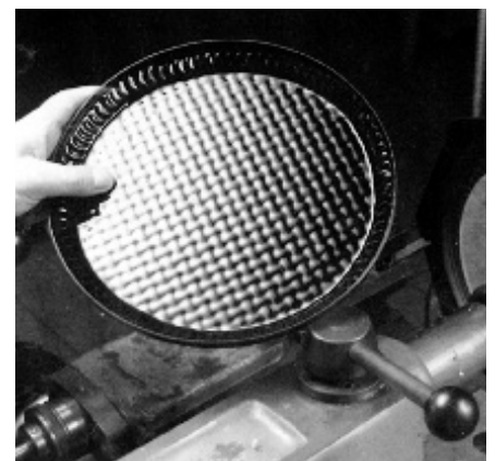
Fig. 34: Cutting off the molded edge
