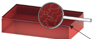
Sheet with UV-protective layer Almost the entire material thickness is UV-sensitive Thin protective layer
